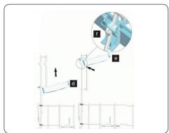
To close the racks, fold them from position (a) to position (b). Make sure the clips on the rack fit on the wire (c). The reverse method can be used to open the racks.
