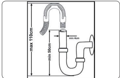
Connect the water drain hose directly to water drain hole or to the sink outlet spigot. This connection should be minimum 50 cm and maximum 110 cm from floor plane.
